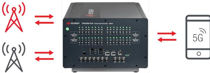
Figure 2. Verifying interoperability with real devices and base stations in the lab
