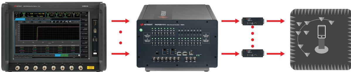
Figure 9. MIMO OTA mmWave testing
