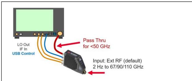
Figure 6: Configuration 1, single input.
