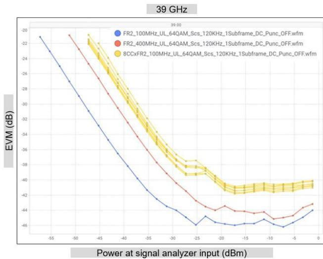
Figure 5. FR2, 39 GHz carrier, CP-OFDM Uplink, 1x100 MHz (blue) and 1x400 MHz (red) and 8x100 MHz (yellow), 64 QAM, 120 kHz SCS
