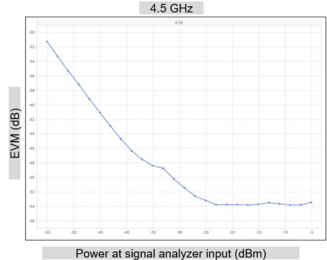
Figure 3. 5G NR FR1, 4.5 GHz carrier, 100 MHz single carrier, 256 QAM, 30 kHz SCS, DC Punc off
